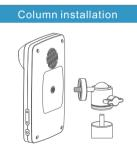
The middle position on the back of this product is inlaid with a standard inch 1/4-inch interface. You can choose the TS-S30 floor stand or use it directly with the standard triangular bracket.
